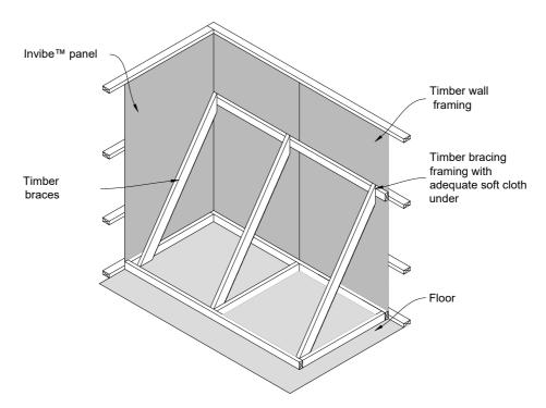
Note: Ensure edges are well braced and timber braces are aligned over solid framing behind
